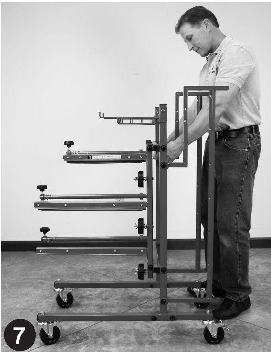
7 Install side frames P/N 500-000. Do not tighten any bolts until all parts are assembled.
