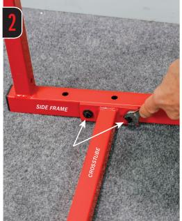
Bolt **Crosstube** to **Side Frame** using 1/4"  $\times$  3/4" bolts and washers. Repeat for opposite side.
