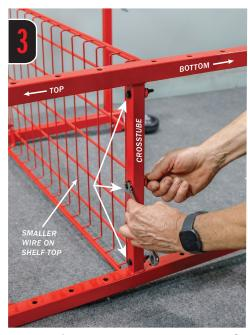
Lay cart flat as shown. Install **Top Shelf** to **Crosstube** using 1/4" x 3/4" bolts and washers. Repeat for opposite crosstube and lower shelf.
