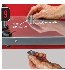
Screw **Tube Connector** into table top until 5/8" shows beneath table. From beneath the table, thread large nut onto tube connector and tighten.
