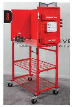
Install **Coupon Tray** and **Tool Tray** in desired locations on **Side Panels.**Bolt **Vise** on using included hardware.
