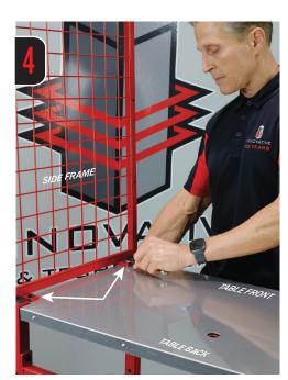
Align upper **Side Frame** and **Table Top** holes as shown and install using 1/4" x 2" bolts and corresponding nuts & washers. Repeat for opposite side.
