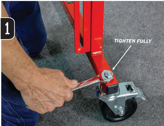
1 Install (4) Total-Lock Caster Wheels into Leg Assembly . Lock wheels as shown.
